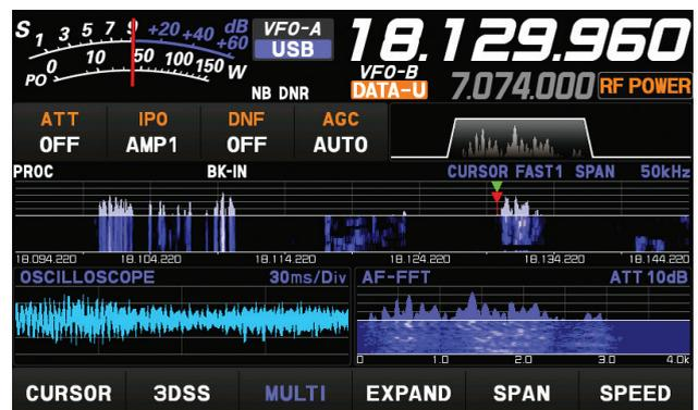
Figure 2 — The FT-710's high-resolution 4.3-inch touchscreen packs a lot of information into a small space.
