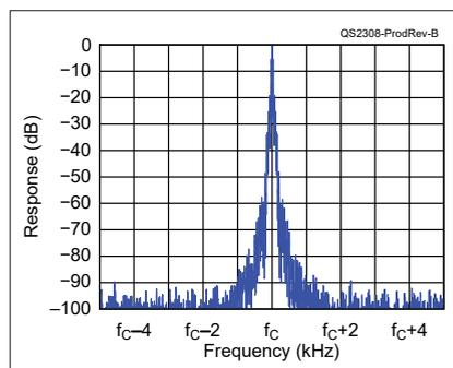
**Figure B** — The spectral display of the Yaesu FT-710 transmitter during keying sideband testing. Equivalent keying speed is 60 WPM using external keying and the default rise time setting. Spectrum analyzer resolution bandwidth is 10 Hz, and the sweep time is 30 seconds. The transmitter was being operated at 100 W PEP output on the 14 MHz band, and this plot shows the transmitter output  $\pm 5$  kHz from the carrier. The reference level is 0 dBc, and the vertical scale is in dB.
