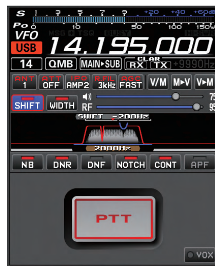
Operating Panel on PC screen
